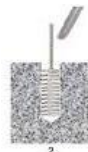
2 Clean Hole By Brushing Or Blowing To Remove All Dust And Debris
